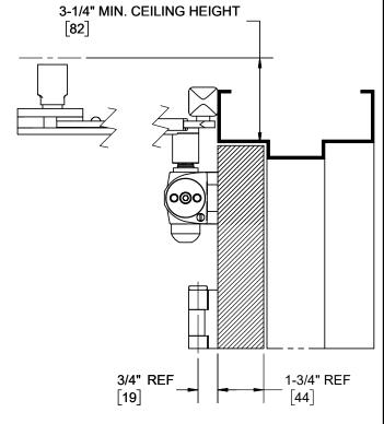
DOOR CLOSER MODELS: 8600 SISH SPRING INTEGRA STOP REGULAR INSTALLATION HOLD OPEN PULL SIDE MOUNT
